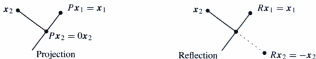
Figure 6.2 Projections have eigenvalues 1 and 0. Reflections have \lambda = 1 and -1 . A typical x changes direction, but not the eigenvectors x_1 and x_2 .
